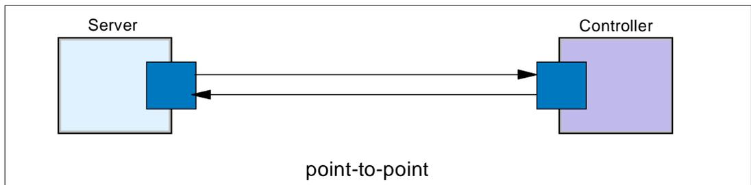
Figure 1 Point-to-point configuration
