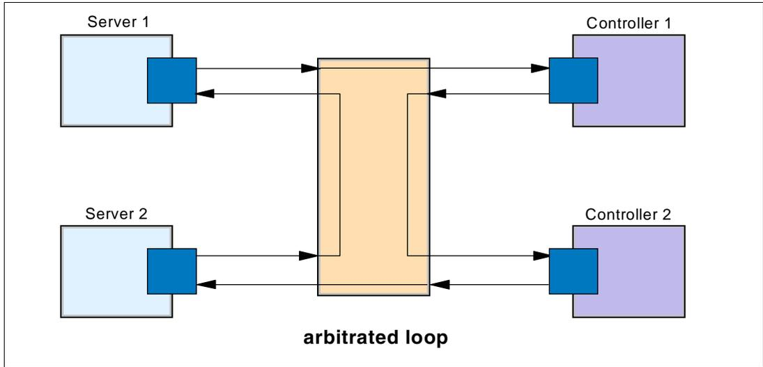
Figure 2 Arbitrated loop configuration
