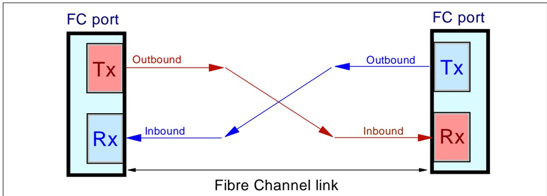
Figure 5 Fibre Channel link
